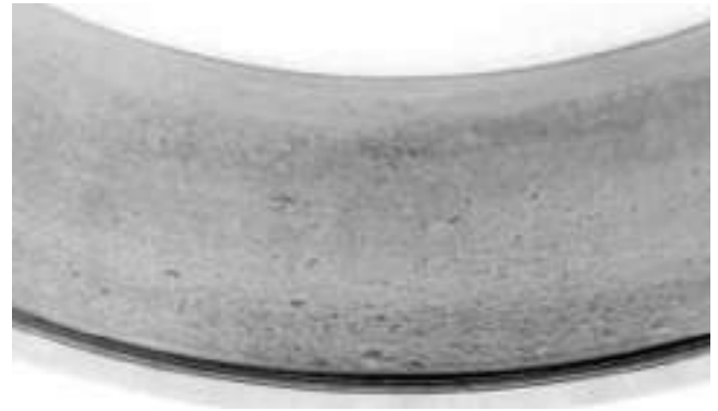
Fig. 160. Bearing damage due to abrasive particles.
