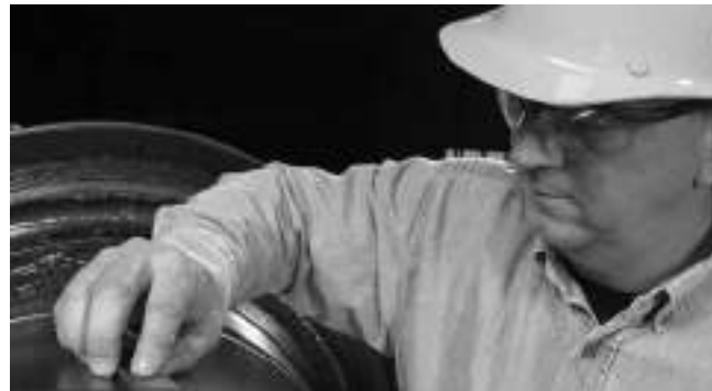
Fig. 240. Restoring minor roll neck damage.
