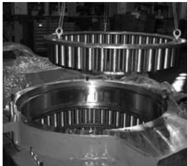
Fig. 230. Handling bearing components with threaded lifting hole.
