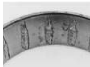
Fig. 191. Deep etching on an outer ring race.
