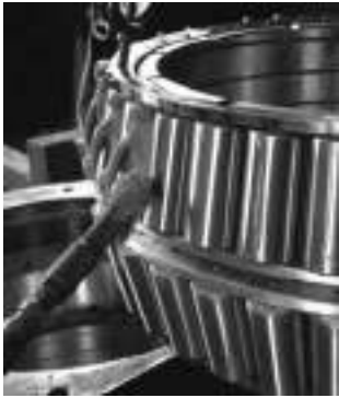
Fig. 245. Lubricating a tapered roller bearing with grease.
