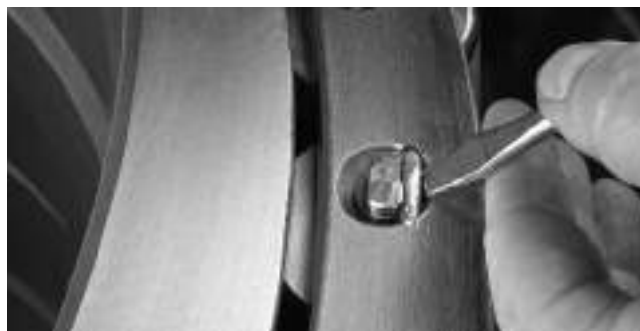
Fig. 231. Removing locking wire from an inspection pin.
