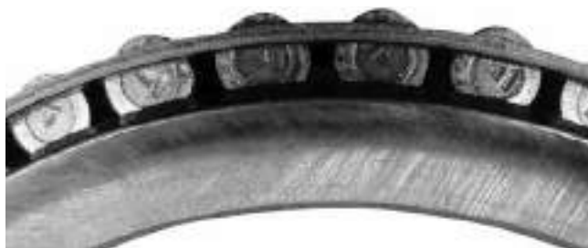
Fig. 183. Roller end and rib discoloration.
