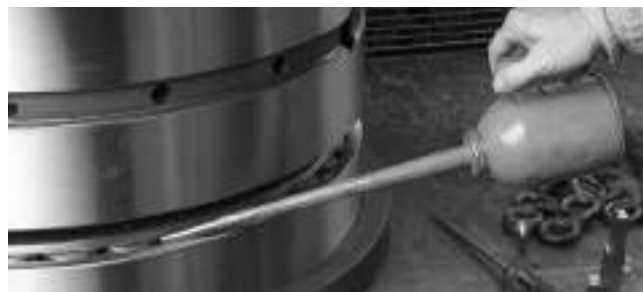
Fig. 267. Applying light oil to rollers and race.
