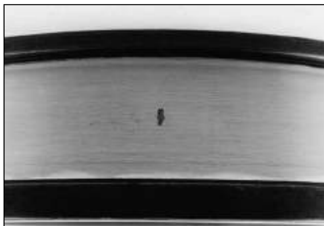
Fig. 169. Inclusion origin spalling.
