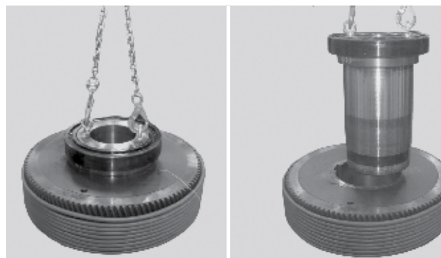
Fig. 204. Example of a 1300 kg (2900 lb.) gear wheel wrapped with two flex coils.
