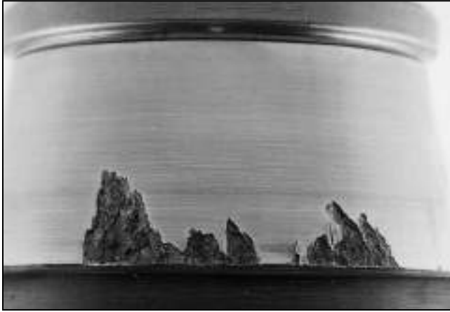
Fig. 171. Geometric stress concentration spalling.
