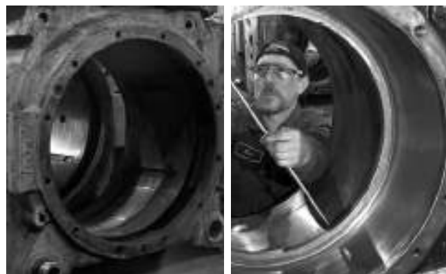
Fig. 278. Chock maintenance before and after photos.
