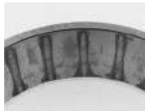
Fig. 189. Staining without pitting.
