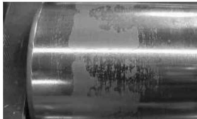
Fig. 184. Roller peeling damage.
