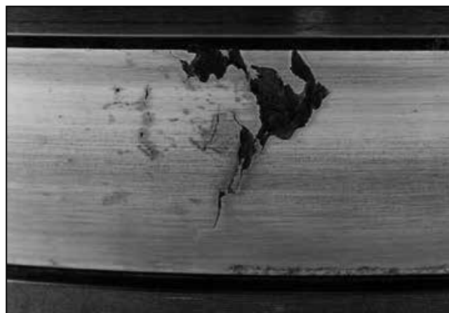
Fig. 170. Point surface origin spalling (PSO).
