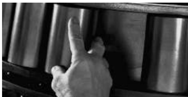
Fig. 233. Inspecting inner race.
